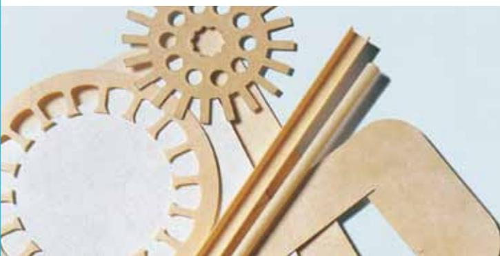
**Type 992** is a low-density pressboard produced in two thicknesses 1.6 and 3.2 mm (63 and 125 mil), with a specific gravity of 0.5. This material's low density allows easy formation of complex shapes and provides the highest saturability of the pressboard products.
