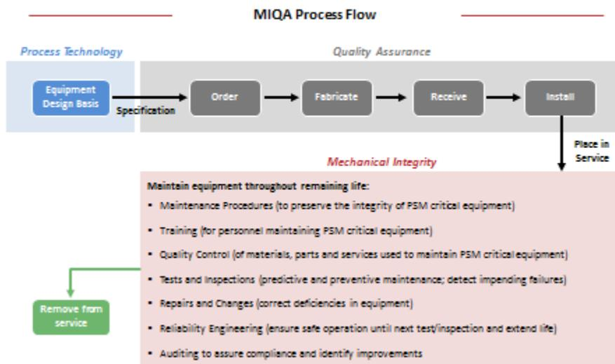
Figure 2 – Tactical aspects of a Mechanical Integrity Barrier
