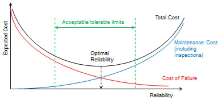
Figure 3 – The Cost Optimised Risk Based approach to tactical inspections in a Mechanical Integrity Program.
